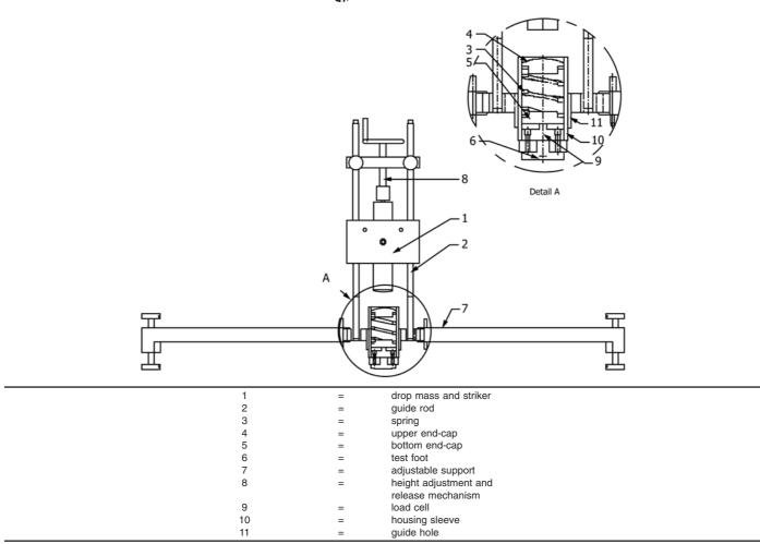
FIG. 1 Force Reduction Test Apparatus
